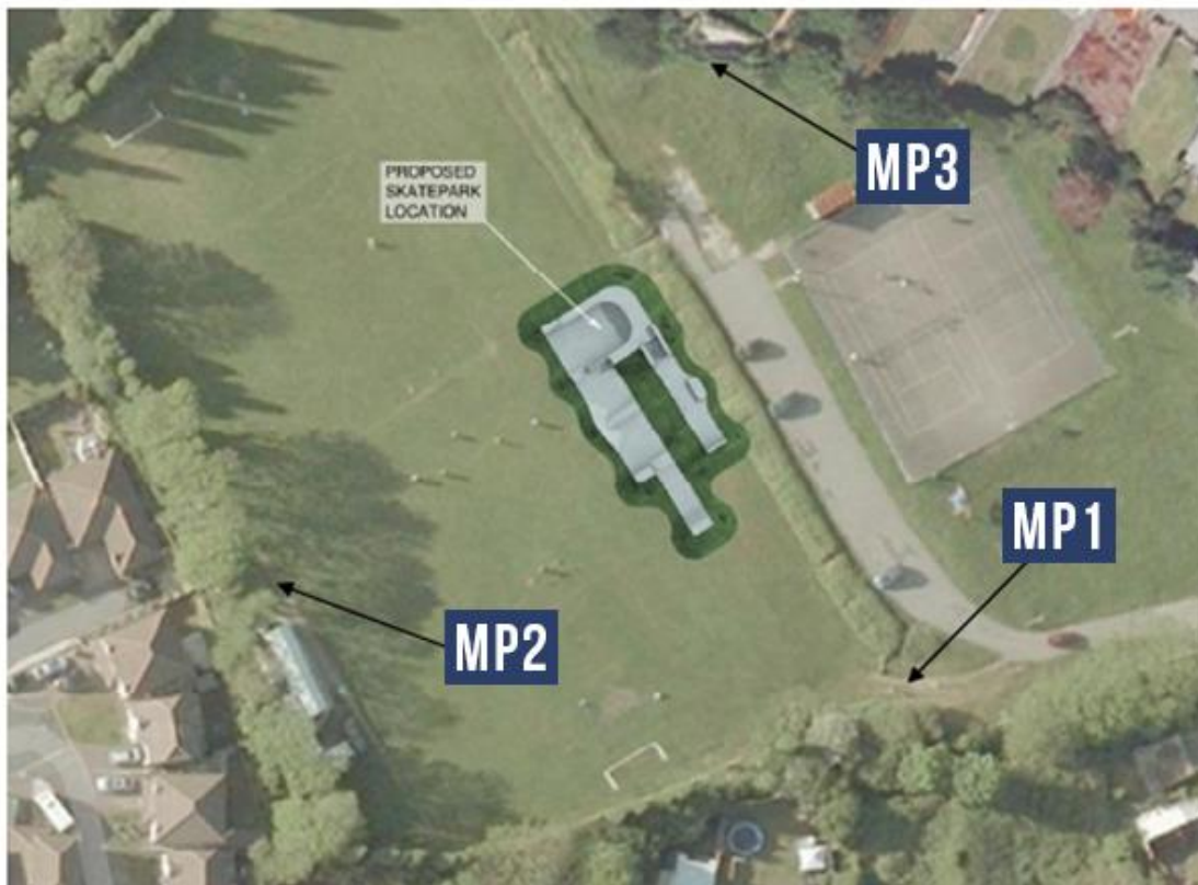
FIGURE 1 - NOISE MEASUREMENT POSITIONS
